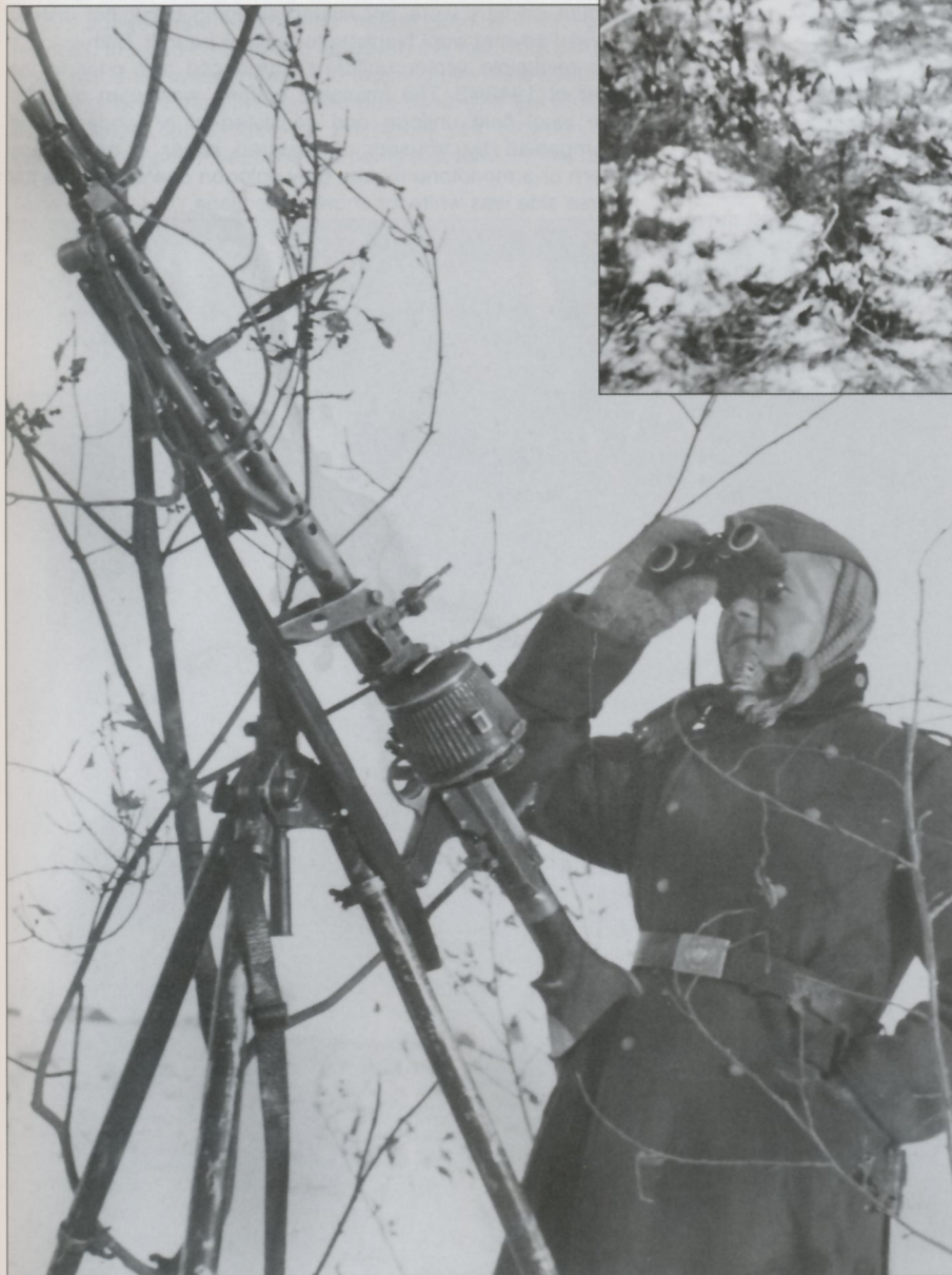
A machine-gunner scans the sky for Soviet aircraft. His MG34, fitted with a 50-round drum magazine and anti-aircraft sights, is set-up on a Dreifuss 34 anti-aircraft tripod mount. The gunner has fastened a non-issue scarf around his head beneath his field cap and wears fur mittens.
