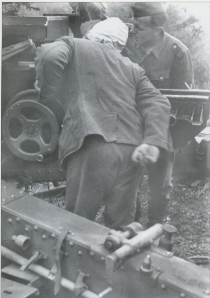
Two artillerymen check the breech of their 15cm s.FH18 heavy field gun prior to bringing it into action, a requirement after transporting it. The Kanonier to the right wears the field grey slip-on unit identification loop on his dark blue-green, red-piped shoulder strap. Previously, unit identification was embroidered in the arm of service color directly on the shoulder straps.
