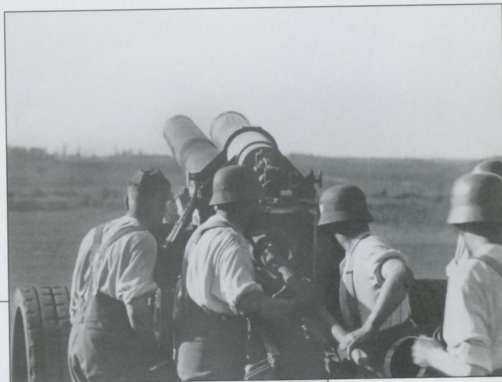
A gun crew rams home a projectile into the breech of a 15cm s.FH18. One of the ammunition numbers holds the cartridge case at the ready, containing the propellant increments. This howitzer belonged to a motorized unit as indicated by its rubber tires. It was hot work, so the crewmen have removed their wool tunics revealing their collarless white shirts. These shirts were quite conspicuous, so later in the war field grey or light grey shirts were issued.
